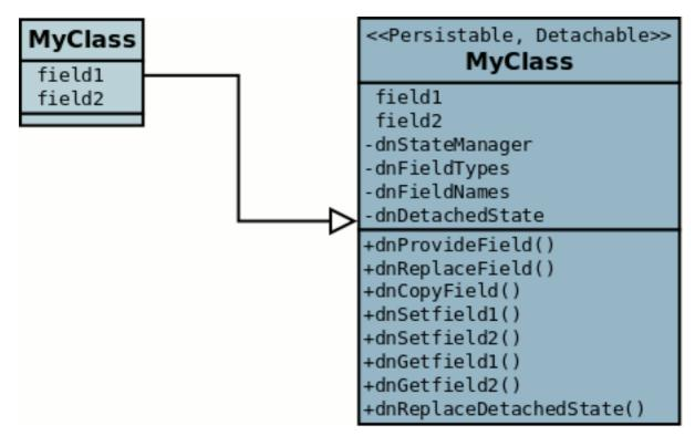
Again, the example above doesn't show all methods added for the Detachable interface but the main thing to know is that the detached state (object id of the datastore object, the version of the datastore object when it was detached, and which fields were detached is stored in "dnDetachedState"). Please see the JDO spec for more details.
