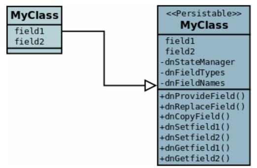
The example above doesn't show all *Persistable* methods, but demonstrates that all added methods and fields are prefixed with "dn" to distinguish them from the users own methods and fields. Also each persistent field of the class will be given a dnGetXXX, dnSetXXX method so that accesses of these fields are intercepted so that DataNucleus can manage their "dirty" state.
