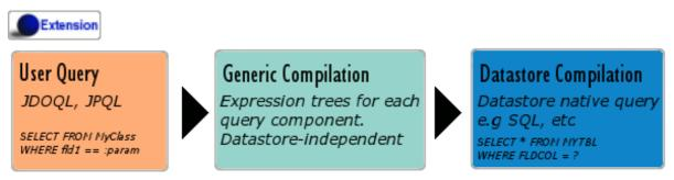
JDO doesn't currently define a mechanism for caching of queries. DataNucleus provides 3 levels of caching
