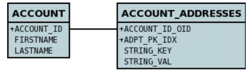
If you want to configure the names of the columns in the "join" table you would use the <key> and <value> subelements of <field> as shown above.
