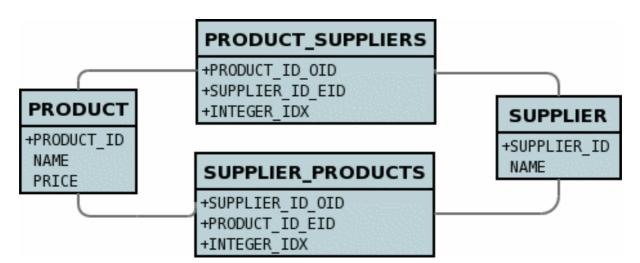
In the case of a List at both ends it doesn't make sense to use a single join table because the ordering can only be defined at one side, so you have to have 2 join tables.
