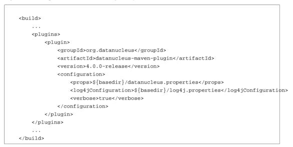
So with these properties when I run SchemaTool it uses properties from the file *datanucleus.properties* at the root of the Maven project. I am also specifying a log4j configuration file defining the logging for the SchemaTool process. I then can invoke any of the Maven goals
