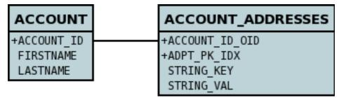
You can configure the names of the key column(s) in the join table using the *joinColumns* attribute of @CollectionTable, or the names of the value column(s) using @Column for the field/method.
