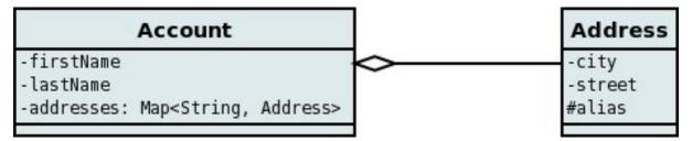
In this relationship, the **Account** class has a Map of **Address** objects, yet the **Address** knows nothing about the **Account**. In this case we don't have a field in the Address to link back to the Account and so DataNucleus has to use columns in the datastore representation of the **Address** class. So we define the MetaData like this
