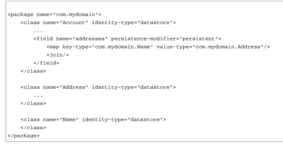
This will create 4 tables in the datastore, one for **Account**, one for **Address**, one for **Name** and a join table containing foreign keys to the key/value tables.
